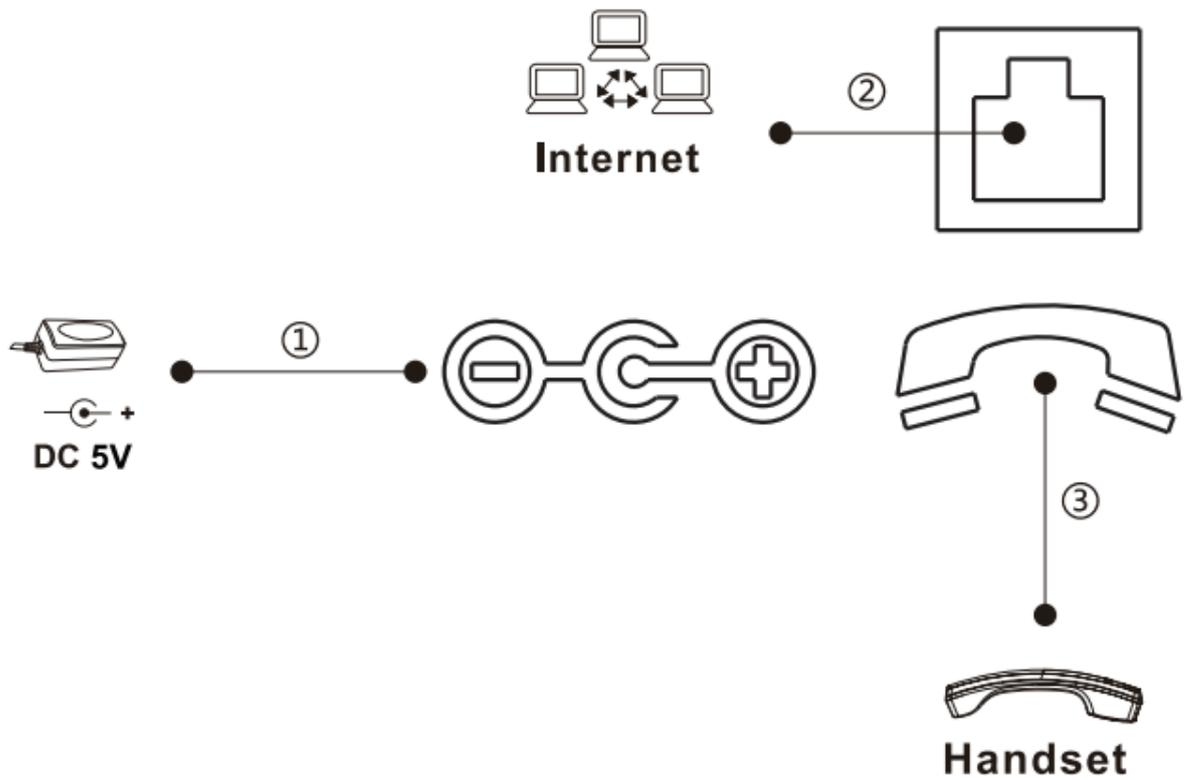
*Figure 2 – Device Connection*
