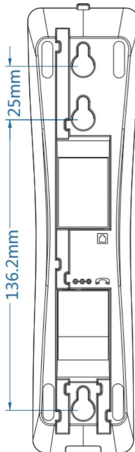
*Figure 1 - Device Installation*
